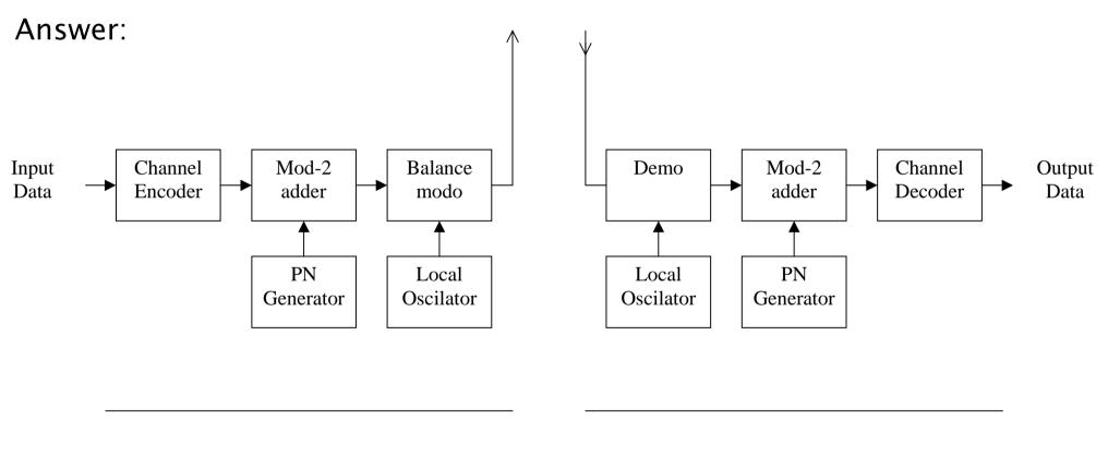
Direct Sequence Transmitter with BPSK
