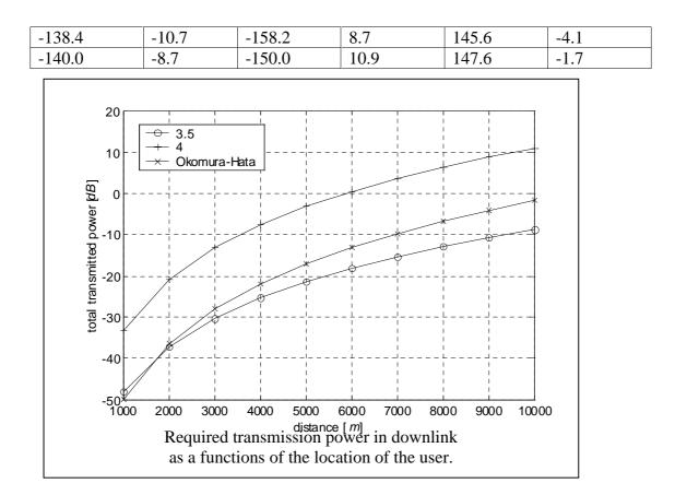
The outage in downlink occurs only if to assume that the attenuation is accordingly attenuation factor 4 and in this case also only if all 10 users are communicating.
