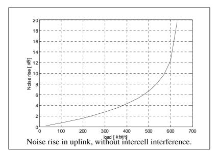
b) The other cell interference can be accounted by scaling the load factor by the intercell interference factor (1 + i).
