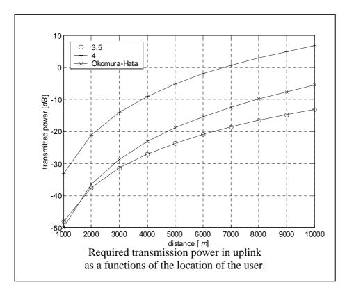
The maximum transmitted power for the handset was limited to the 0.1 W (-10 dB). Because of that limit we see if the attenuation in the channel follows the attenuation law -4 the users farther than 7000 m are all in the outage i.e. they do not have enough power to be connected to the BS.
