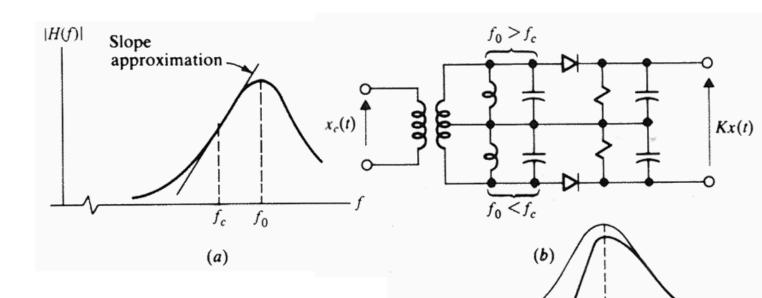
a) slope detector realized by tank-circuit
