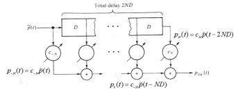
Search for the tap gains  $c_N$  such that the output equals zero at sample intervals D except at the decision instant when it should be unity. The output is (think for instance paths  $c_{-N_0}$   $c_N$  or  $c_0$ )
