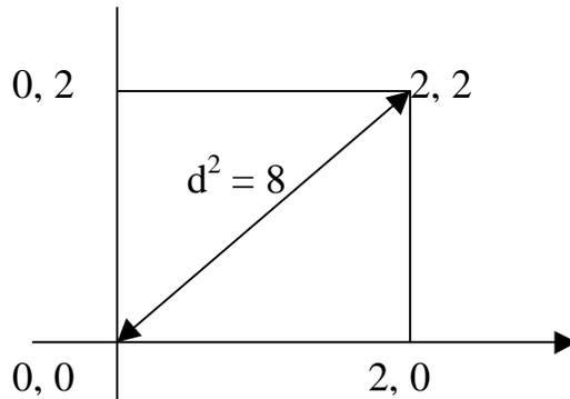
Since these are four possible two-signal sequences but only two successor states for  $s_0$  - i.e  $s_0, s_1$  there will be parallel transitions. The two signal sequences are partitioned into pairs such that the inter-sequence distance in each pair is maximized.
