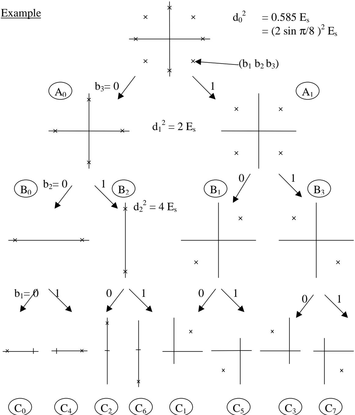
Set partitioning of 8-PSK with associated bit labeling
