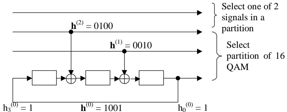
It is shown that the number of coded bits, 2, remains unchanged for most of MPSK, MQAM schemes regardless of the memory and signal points. This is for best TCM codes in AWGN channel.
