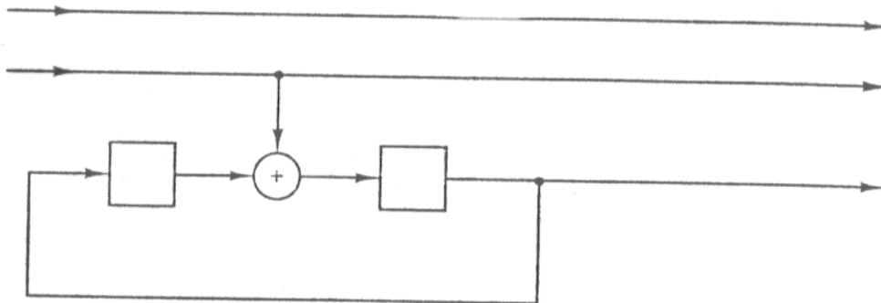
Four-state encoder for 8-PSK in systematic form with feedback.
