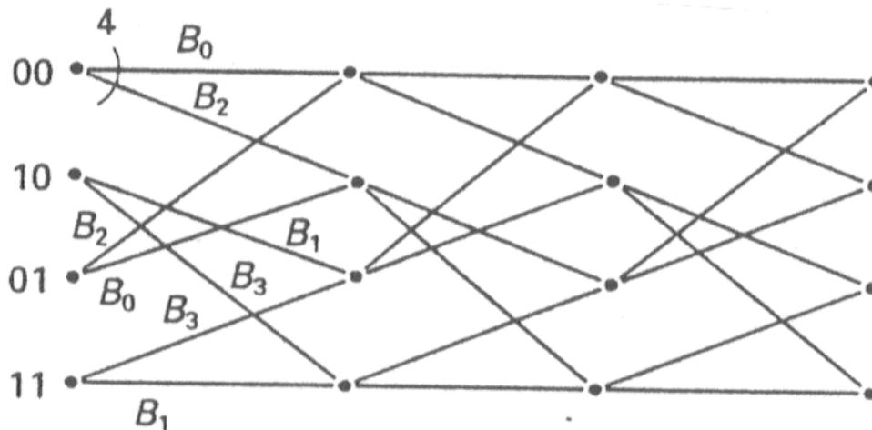
Trellis labeling for 4-state, 8-PSK code. Subsets have size 2.
