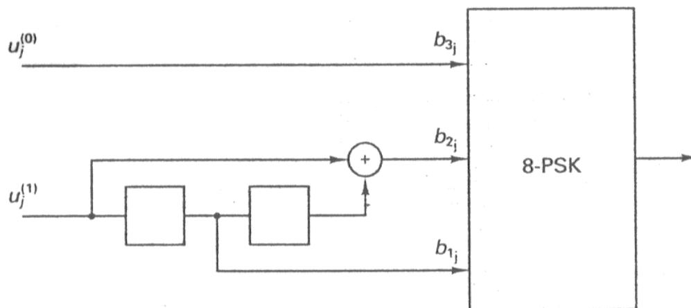
Feedforward encoder realization of best 4-state code for 8-PSK.
