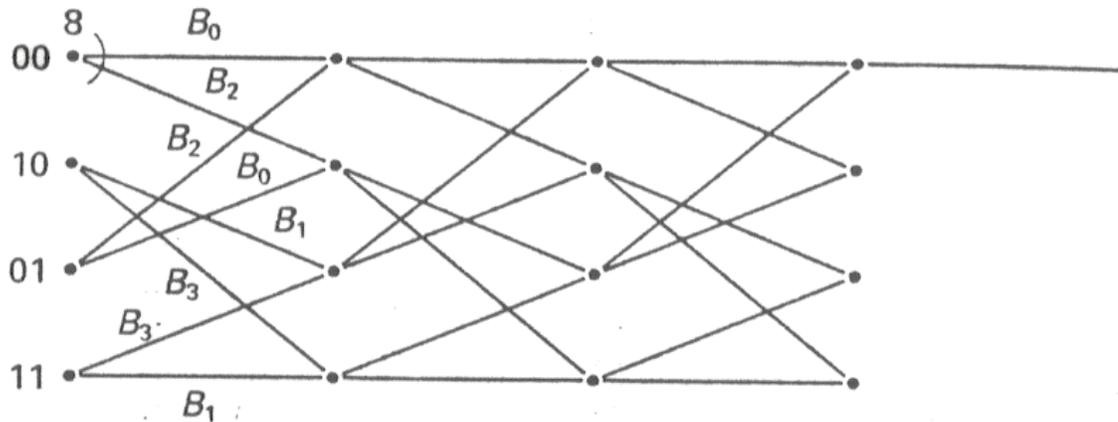
Trellis labeling for 4-state, 16 QAM code. Note similarity with 4-state, 8-PSK design. Subsets have size 4.
