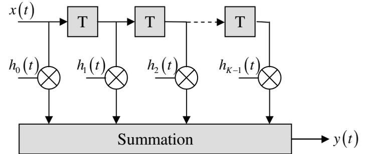
Figure 6 Tapped delay line presentation of a wideband multipath radio channel
