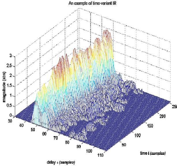
Figure 2 Example of measured impulse response in Tapiola Espoo, frequency is 2 GHz
