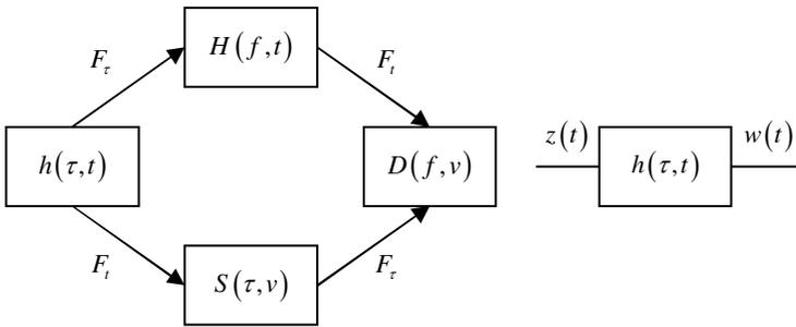
Figure 3 Relationships between deterministic system functions of an LTV-channel.
