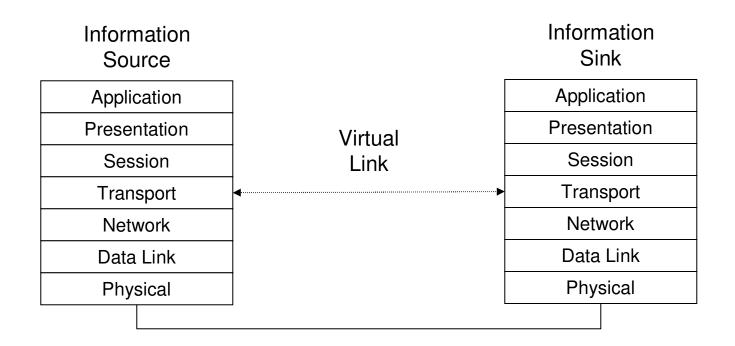
Seven layers of OSI a model of communications
