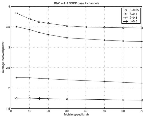
Fig. 10. Average received power as function of mobile speed for algorithm [3]
