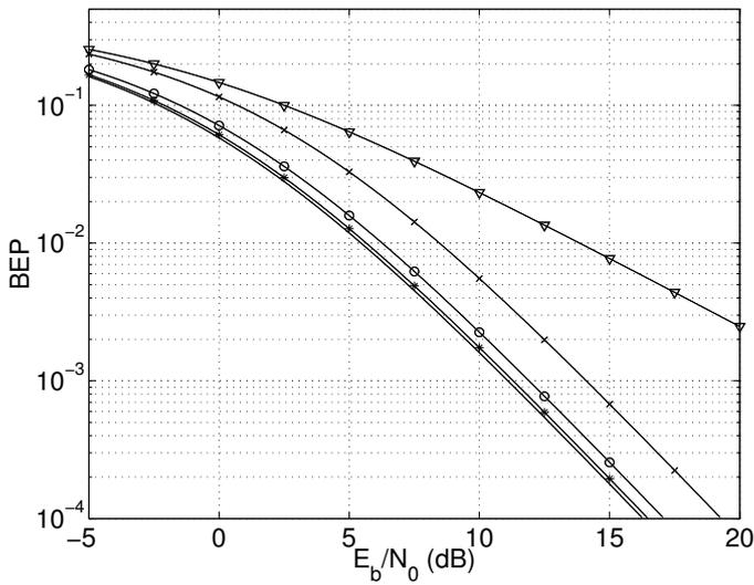
Fig. 4. Performance comparison between Mode 1 (-o-), Mode 2 (-\*-) and Space-Time Transmit Diversity (STTD) (-x-) and single antenna transmission (-∇-). System is 2x1, feedback delay is neglected, channel is block fading for STTD (source: [6] and courtesy of authors).
