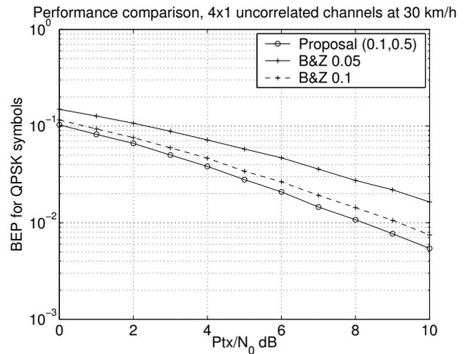
Fig. 8. Bit Error Rate curves for 4x1 uncorrelated channels at 30 km/h. “B&Z” refers to [3], proposal’s parameters are given as  $(\beta, \lambda_G)$  and refer to [5].
