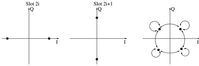
Fig. 2. Weight calculation at BS for Mode 1, with filtering over two slots
