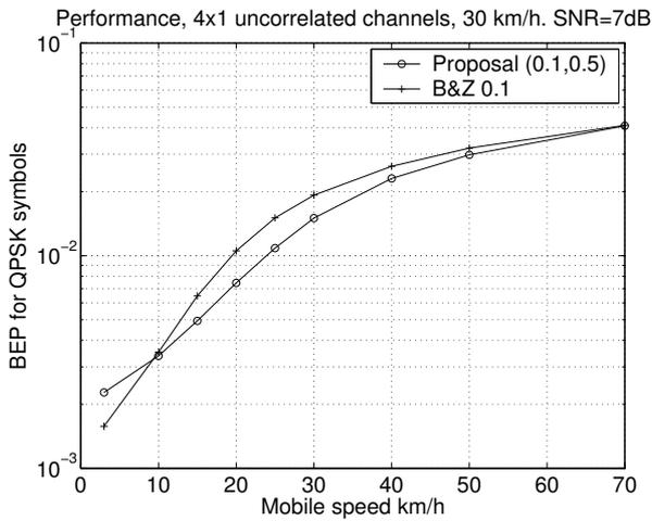
Fig. 9. Bit Error Rate as function of speed in 4x1 uncorrelated channels. "B&Z" refers to [3], proposal's parameters are given as  $(\beta, \lambda_G)$  and refer to [5]. Transmit power to noise power ratio is 7 dB.
