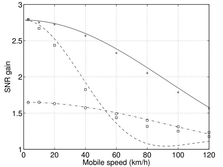
Fig. 6. Received power with adaptive transmit beamforming, 4% feedback errors. (o) and (-) represent Mode 1 (simulation and theoretical result, respectively), cophase algorithm (extension to Mode 1,  $N_T = 4$ ) at 1500 (-) (simulations: □) and 4500 bps feedback rate (-) (and simulated (x)). Source: [6] and courtesy of authors.
