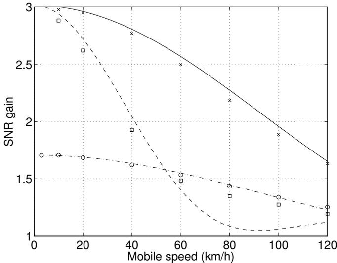
Fig. 5. Received power with adaptive transmit beamforming, no feedback errors. (o) and (-) represent Mode 1 (simulation and theoretical result, respectively), cophase algorithm (extension to Mode 1,  $N_T = 4$ ) at 1500 (-) (simulations: □) and 4500 bps feedback rate (-) (and simulated (x)). Source: [6] and courtesy of authors.
