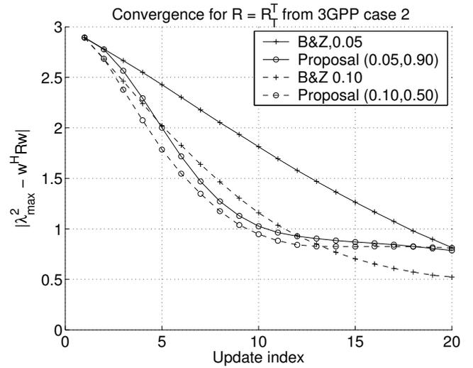
Fig. 7. Convergence in static channel. “B&Z” denotes the algorithm in [3]. Filtered gradient converges uniformly faster when same convergence step ( $\beta$ ) is used, up to the point where learning curves cross. Filtered gradient’s parameters are given as  $(\beta, \lambda_G)$ .  $\lambda_{\max}^2$  is the dominant eigenvalue of  $\mathbf{R}$ . “Proposal” refers to [5].
