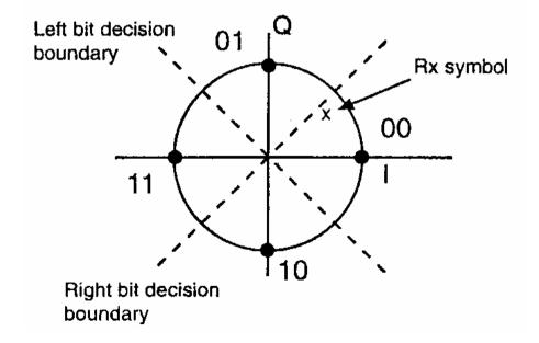
Soft decision: Output of the modulator retains information about the reliability of the decision. The reliability of the detected bits coded in the absolute value of the bits. The absolute value is the distance to the decision boundary.
