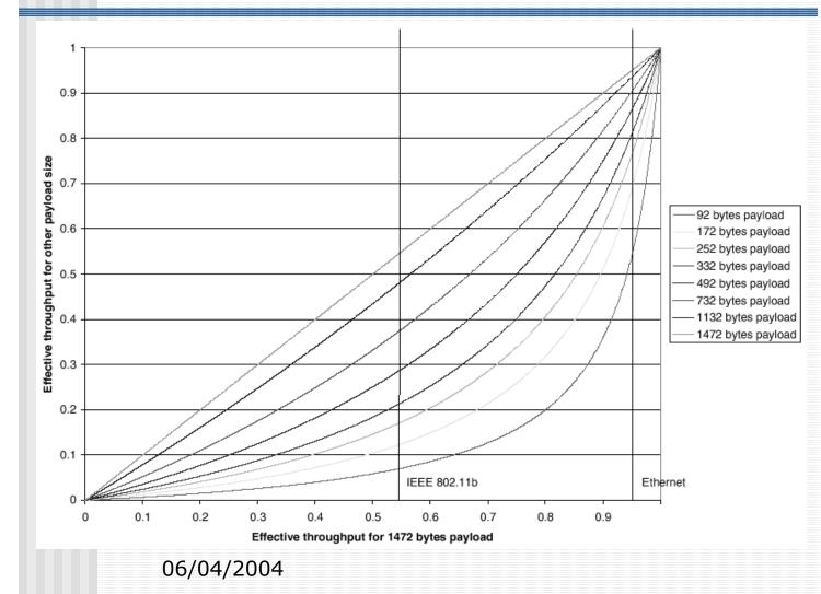
Effective throughput of a network for 92, 172, 252, 332, 492, 732, 1132 and 1472 bytes (packet sizes used by a G711 a-Law codec with audio data length 10ms, 20ms, 30ms, 40ms, 60ms, 90ms, 140ms, respectively) of payload as a function of the effective throughput for 1472 bytes of payload. The vertical lines mark the values for IEEE 802.11b and Ethernet.
