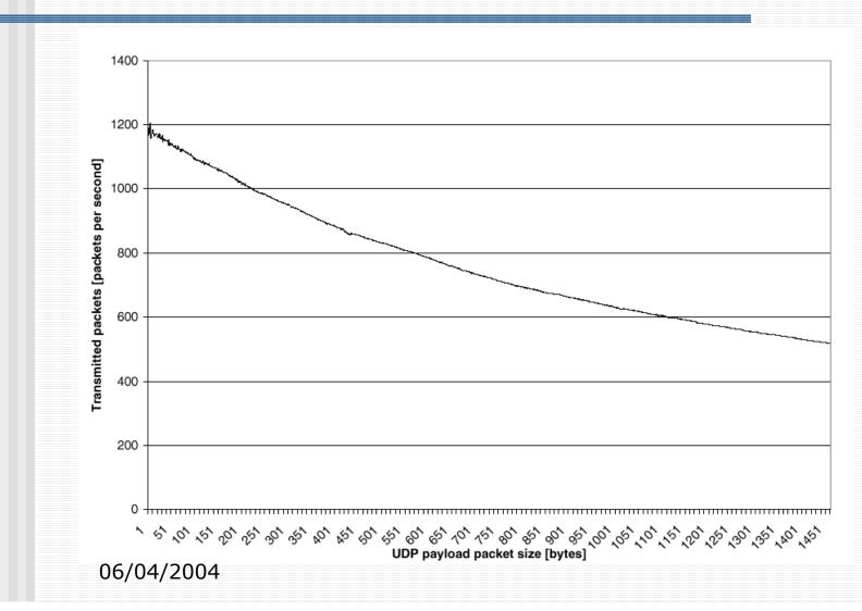
Maximal number of VoIP connections using ITU G711 A-LAW codec
