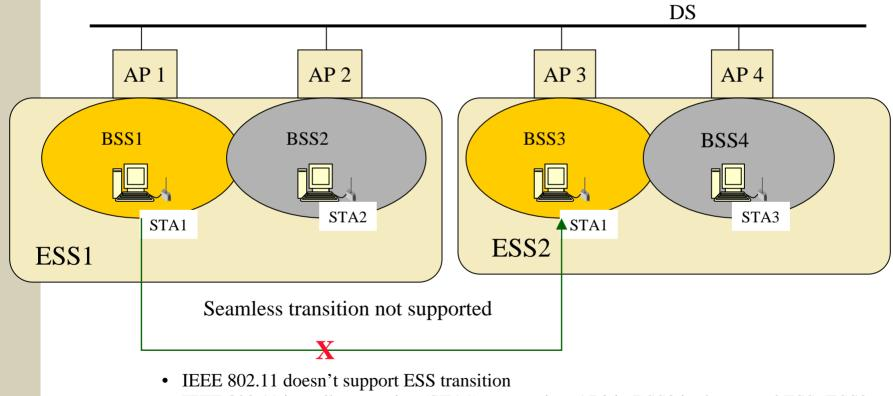
• IEEE 802.11 just allows station (STA1) to associate AP3 in BSS3 in the second ESS (ESS2, when it has first left the first ESS (ESS1)
