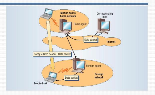
Mobile IP transmission: A corresponding hosts sends an IP data packet to a mobile host. Packet is tunneled from the mobile host's home network to its current foreign network.
