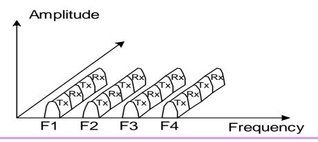
Radio network topology and fixed assignment channel access method
