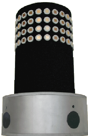
SPUCPA: Stack Polarimetric Uniform Circular Patch Array, N=96 elements.
