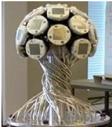
PSSPA: Polarimetric Semi-Spherical Patch Array, N=21 elements.
