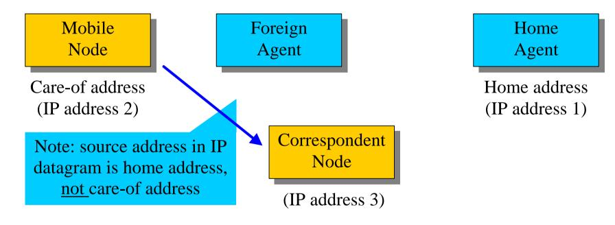
Mobile node sends IP datagram directly to correspondent node (no tunneling required)
