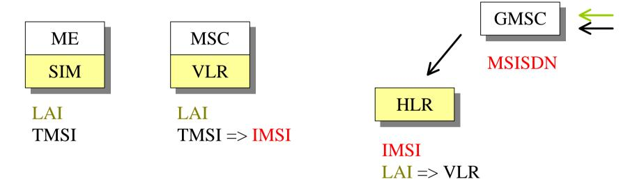
MTC is directed through PSTN to GMSC using MSISDN. GMSC contacts HLR (MSISDN in fact points to the HLR database of this subscriber containing IMSI, LAI, etc.)
