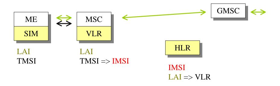
Only the mobile subscriber with the correct TMSI reacts to the paging. A connection between MS and MSC is established and the call set-up is completed.
