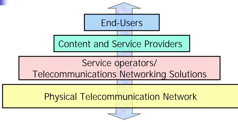
Telecommunication network content and technology producers, operators and consumers form an interoperable hierarchy
