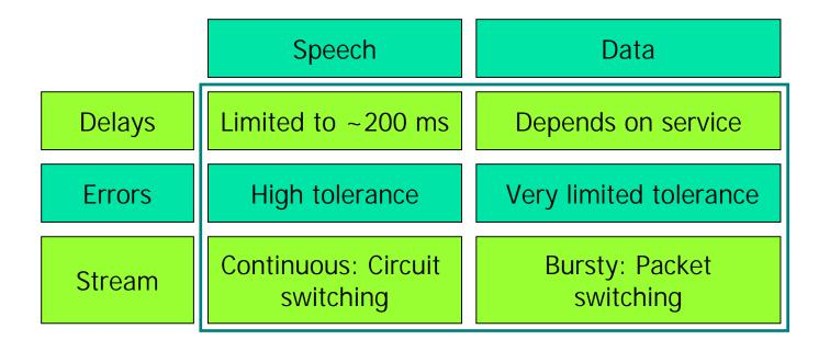
Teletraffic can be forced to fixed rate or bandwidth as speech in PSTN or in ATM traffic (->waste of network resources)
