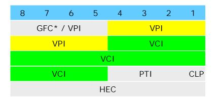
VPI and VCI are virtual connection identifiers (used for switching or relaying the cells to the correct destination)
