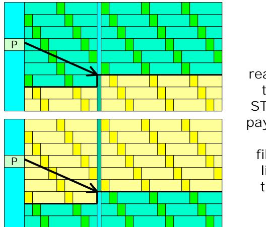
In reality, the STM-1 payload is filled like this
