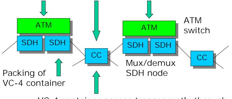
VC-4 container passes transparently through SDH cross-connect (CC) equipment
