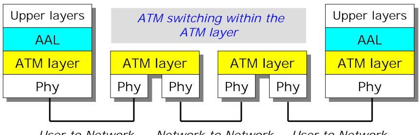
User to Network Interface (UNI) Network to Network Interface (NNI) User to Network Interface (UNI) ATM is a transport technique for implementing network "backbone"
