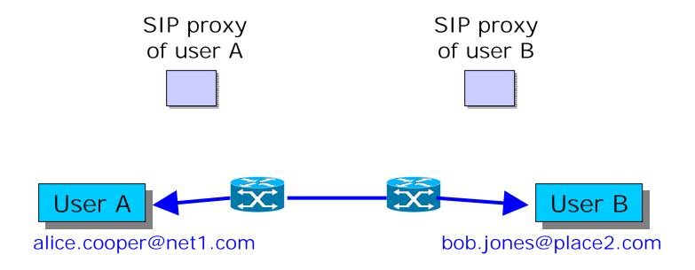
After successful session establishment, the user plane data (e.g. coded speech carried on top of RTP) is carried between the terminals directly through the Internet without involving SIP proxies.
