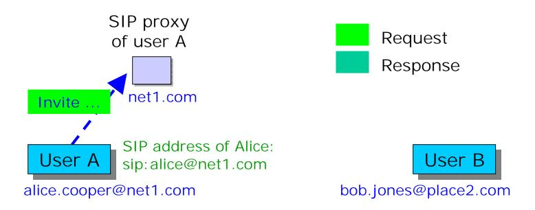
"Invite" message (corresponding to IAM message in ISUP) is sent to SIP proxy of user A. The message includes SIP address (sip:bob@net2.com) of user B.
