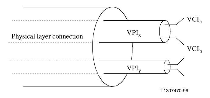
NOTE –  $VCI_a$  and  $VCI_b$  represent two of the possible values of VCI within the VP link with the value  $VPI_x$ . Similarly,  $VPI_x$  and  $VPI_y$  refer to two of the possible values of VPI within the physical layer connection.
