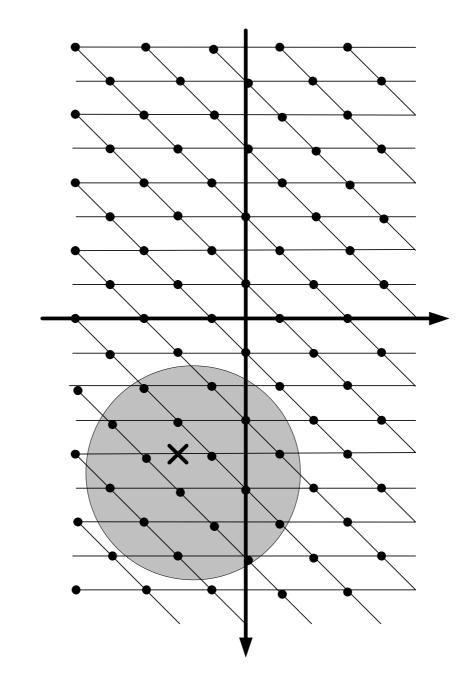
Figure 17: Points considered in a sphere decoder.
