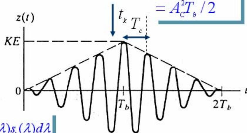
$$\int_0^{T_b} [s_1(\lambda) - s_0(\lambda)]^2 d\lambda = \underbrace{\int_0^{T_b} s_1^2(\lambda) d\lambda}_{E_1} + \underbrace{\int_0^{T_b} s_0^2(\lambda) d\lambda}_{E_0} - 2 \underbrace{\int_0^{T_b} s_0(\lambda) s_1(\lambda) d\lambda}_{E_{10}}$$
