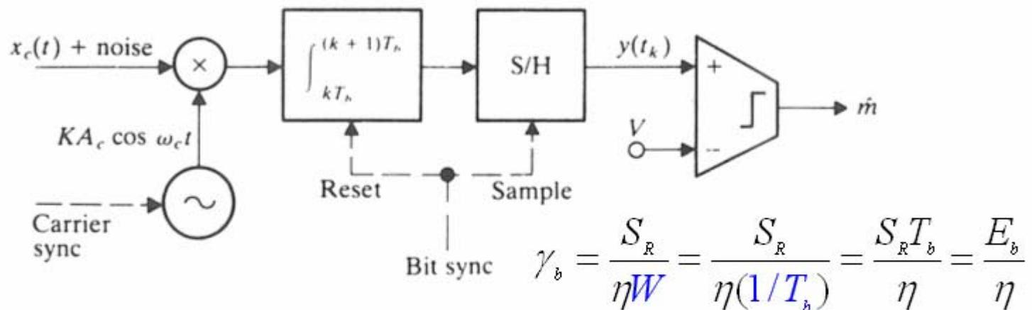
$$E_1 = \int_0^{T_b} s_1^2(\lambda) d\lambda = A_c^2 T_b / 2, \quad E_0 = 0, \quad E_{10} = \int_0^{T_b} s_1(\lambda) s_0(\lambda) d\lambda = 0$$
