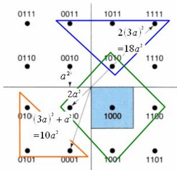
$$p_e = 3Q\left(\frac{a}{\sigma}\right) = 3Q\left(\sqrt{\frac{\overline{A^2}}{10\sigma^2}}\right) = 3Q\left(\sqrt{\frac{2E}{10N_0}}\right) \text{ symbol error rate}$$
