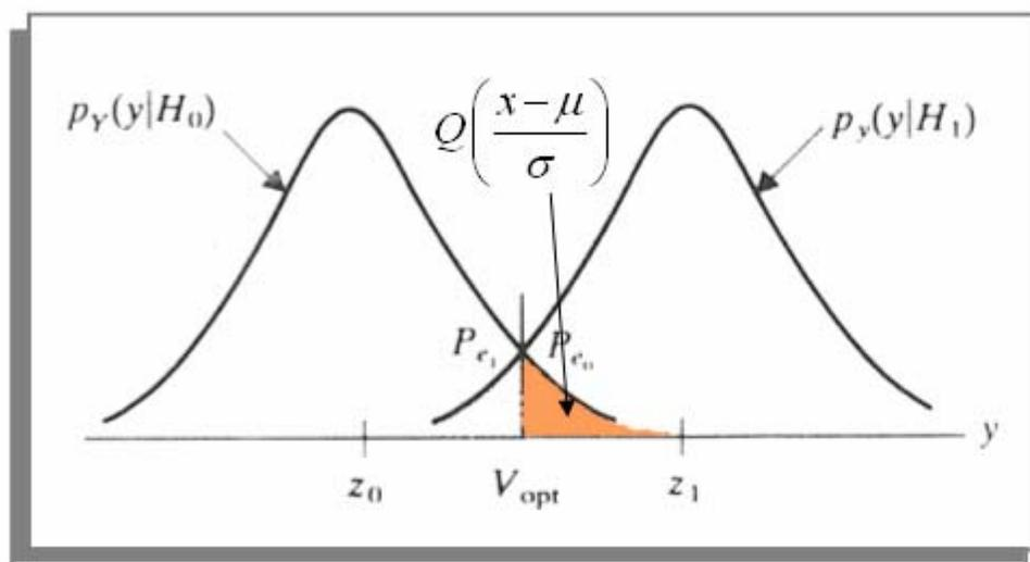
For optimum performance we have the maximized **SNR** that is obtained by matched filtering/integrate and dump receiver
