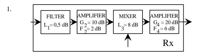
The figure shows the block diagram of a radio receiver and the noise figures and gains of the different blocks. The filter and mixer temperatures are 290 K.
