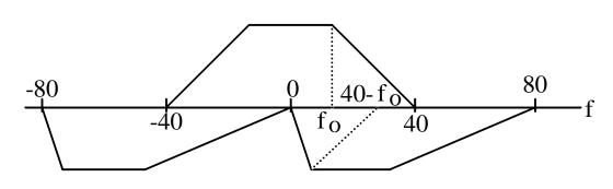
The channel spacing in a radio relay system is 40 MHz, the transmission rate in a channel is  $2 \times 155,52$  Mbit/s + 5% from the radio frame. The total matched filtering gives the trapezoidal pulse spectrum shown in the figure.
