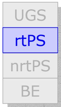
The Real-time Polling Service (rtPS) is designed to support real-time service flows that generate variable size data packets on a periodic basis, such as VoIP (with silence suppression) or streaming video.
