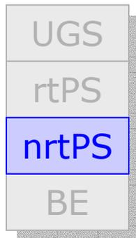
The Non-real-time Polling Service (nrtPS) is designed to support non-real-time service flows that require variable size bursts in the uplink on a regular (but not strictly periodic) basis.
