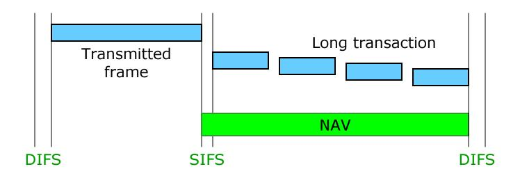
Virtual carrier sensing using NAV is important in situations where the channel should be reserved for a "longer time" (RTS/CTS usage, fragmentation, etc.).
