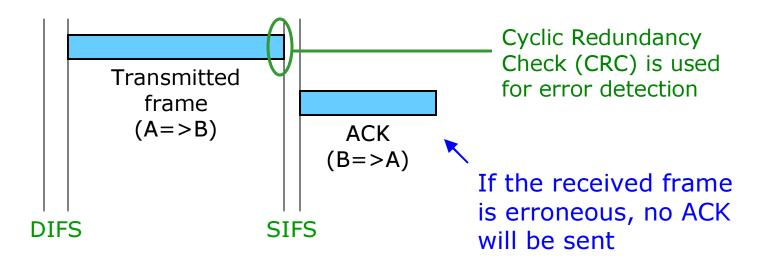
When a frame is received without bit errors, the receiving station (B) sends an Acknowledgement (ACK) frame back to the transmitting station (A).
