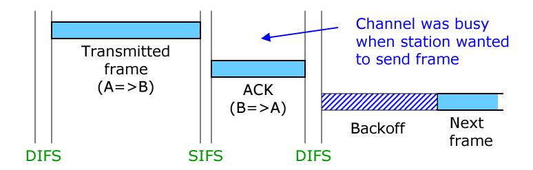
When a station wants to send a frame and the channel is busy => the station must wait a backoff time before it is allowed to transmit the frame. Reason? Next two slides...
