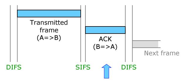
There are two mechanisms for reserving the channel: Physical carrier sensing and Virtual carrier sensing using the so-called Network Allocation Vector (NAV).
