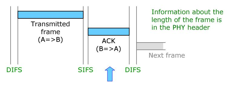
Physical carrier sensing means that the physical layer (PHY) informs the MAC layer when a frame has been detected. Access priorities are achieved through interframe spacing.
