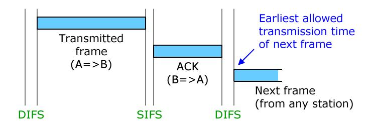
During the transmission sequence (Frame + SIFS + ACK) the medium (radio channel) is reserved. The next frame can be transmitted at earliest after the next DIFS period.
