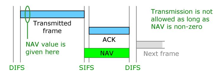
Virtual carrier sensing means that a NAV value is set in all stations that were able to receive a transmitted frame and were able to read the NAV value in this frame.
