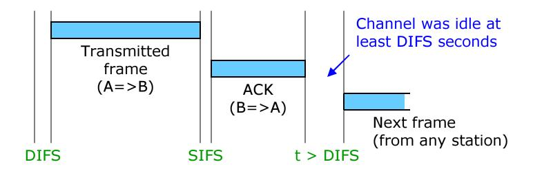
When a station wants to send a frame and the channel has been idle for a time > DIFS (counted from the moment the station first probed the channel) => can send immediately.
