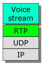
Time stamps can be used at the destination to ensure synchronised play-out of (e.g.) voice samples.
