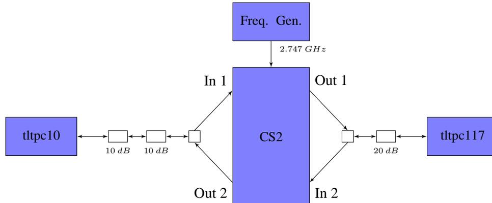
Make the measurements for two different packet sizes 300 and 1470. Set tltpc10 to be server and tltpc117 to be client. Make measurements for relevant channel attenuation values (the values where the throughput changes) such that you can present the result on the plot.
