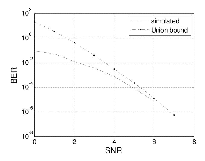
Calculate the union bound for a Viterbi equalizer in a two tap channel.
