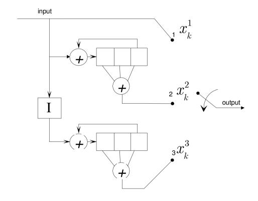
The bit sequence at the interleaver output is  $d_k = \begin{bmatrix} 1 & 0 & 1 & 0 & 1 & 0 & 0 & 1 \end{bmatrix} \Rightarrow d_{i,k} = \begin{bmatrix} 1 & 0 & 0 & 0 & 1 & 0 & 1 \end{bmatrix}$
