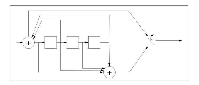
The encoder starts from zero state, collects three bits and adds to them a parity bit calculated based on the previous state and the bit values. The information bits and parity bits are transmitted. In next interval the process is repeated but the initial state is equal to parity bit value in the next interval. Draw the trellis for given code. (This type of code is called zigzag code).
