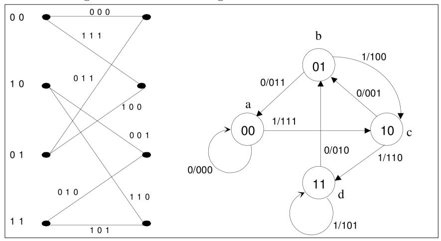
Decoding example: Decode the message using hard decision Viterbi algorithm.
