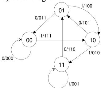
c) Modified state diagram indicating the weights of transitions (node 00 split into two):
