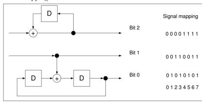
Given the trellis encoder on the figure above.
