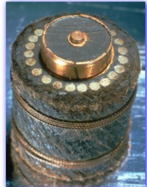
Figure: Cross-sectional view of the TAT-1 cable 1956 (Source: National Museum of American History)
