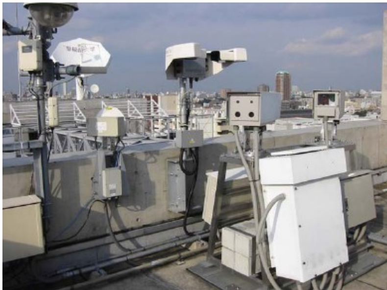
Figure: Rooftop FSO installation
