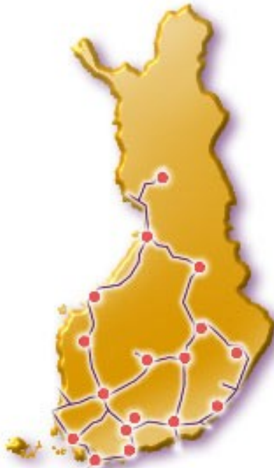
Figure: Corenet's 5800 km mostly fiber backbone network laid along VR railway lines
