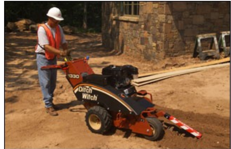
Figure: Compact walk-behind trencher (Source: Ditch Witch).
