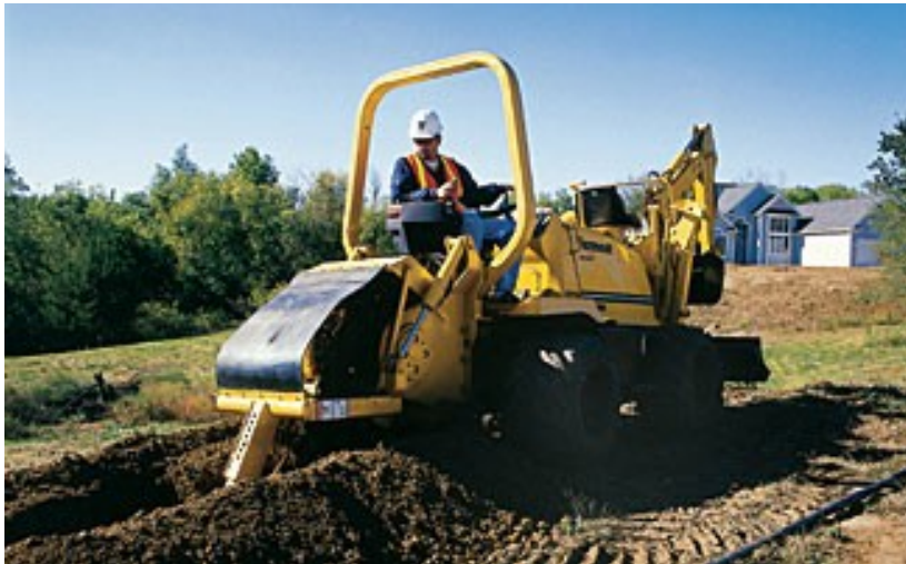
Figure: Heavy duty ride-on trencher (Source: Vermeer).
