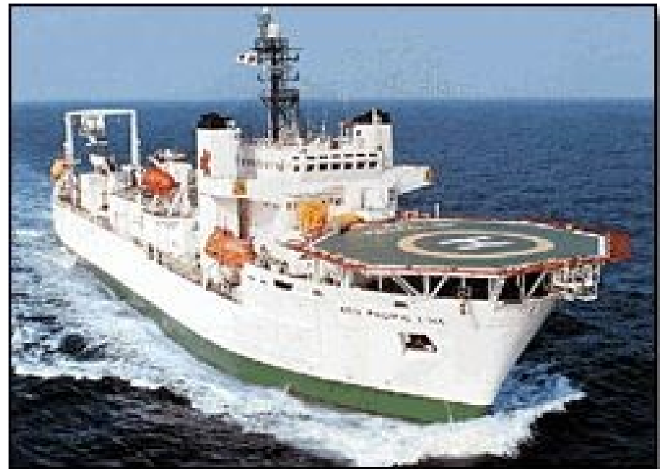
Figure: Cable installation and maintenance ship (KDD, Japan)
