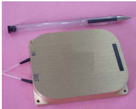
Figure: A compact mini EDFA module. Single function: amplify WDM signal.
