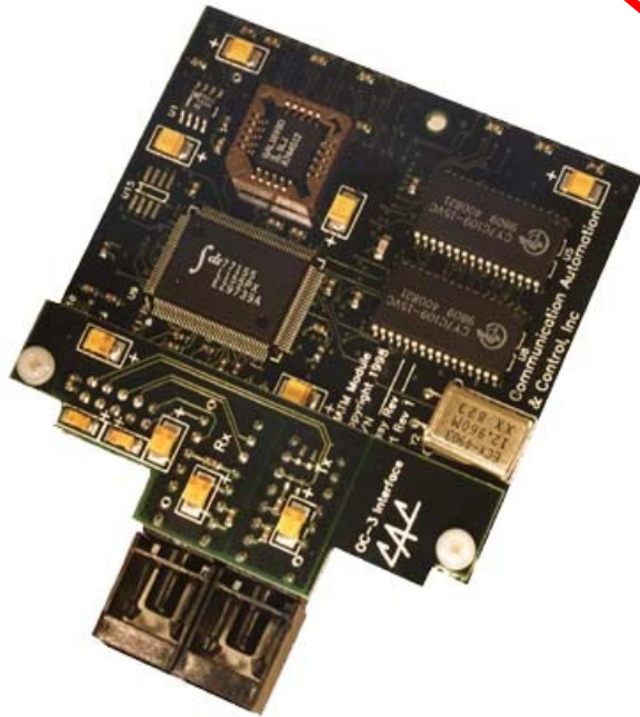
Example: An OC-1/OC-3/STM-1 ATM-SDH/SONET interface module (by Communication Automation Corporation )
